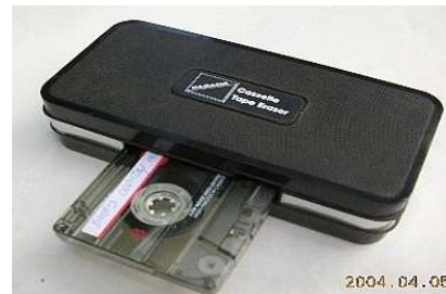
This is a cassette tape demagnetiser where one pushes the cassette through the unit a couple of times.
